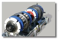
High-pressure gas lines must comply with the highest safety standards meaning that every weld seam has to be perfect. That's why operating companies such as terranets bw GmbH regularly inspect wall thickness in pipes using pipeline inspection gauges, also known as "pigs".
