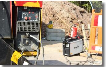
quired are easy to handle, compact and suitable for use on building sites. The Degauss 600 is easy to use and, thanks to the remote control, the power source can even be placed outside the excavation. The dream team: EWM power source PICO 260 CEL PWS and the Degauss 600 (in the background)
